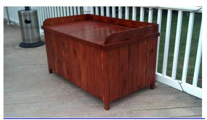
Cedar chest I made. Unfortunately, even using a nice UV protective spar urethane, the lids warped in the sun.
